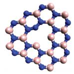
**Figure 2:** Molecular structure of the  $N_BV_N$  defect within the hBN lattice (Tran et. al., 2015).
