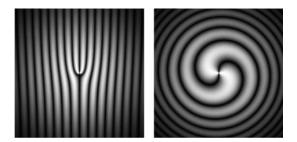
(**b**) Theoretical interference patterns for planar (left) and spherical (right) phase provided by Carpentier et al. (2008).
