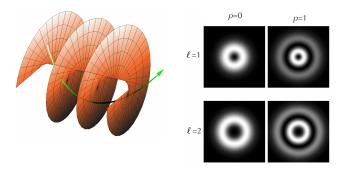
**Figure 1:** Surface of constant phase around an optical vortex; the Poynting vector is shown in green [9].
