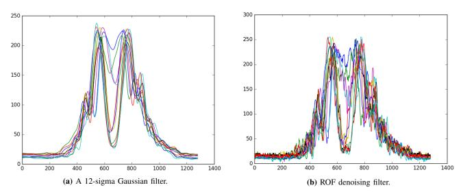
Figure 9: Above are several intensity profiles for x slices of an observed optical vortex for both Gaussian filtering and ROF denoising.
