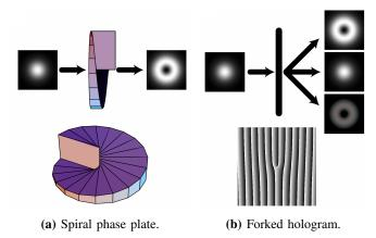
**Figure 3:** Two methods of producing an optical vortex using a machined spiral phase plate or a forked hologram with a blazed diffraction grating (O'Holleran, 2008).
