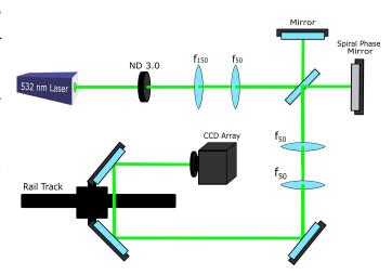
Figure 4: The experimental set up which was used to analyse the various characteristics of optical vortices.
