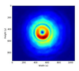
Figure 5: A charge 2 optical vortex after image smoothing.
